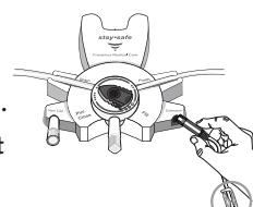
8. Remove protective cap from stay•safe DISC and set aside.
