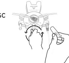
9. Connect stay•safe catheter extension set to the stay•safe DISC.
