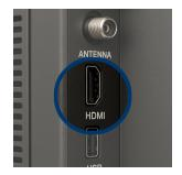
Plug the HDMI cable into the "TO TV" port. Then, connect the other end to your television's HDMI input.
